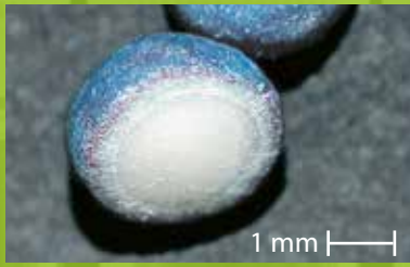
Cellets 1000 coated Stereomicroscopic shot
